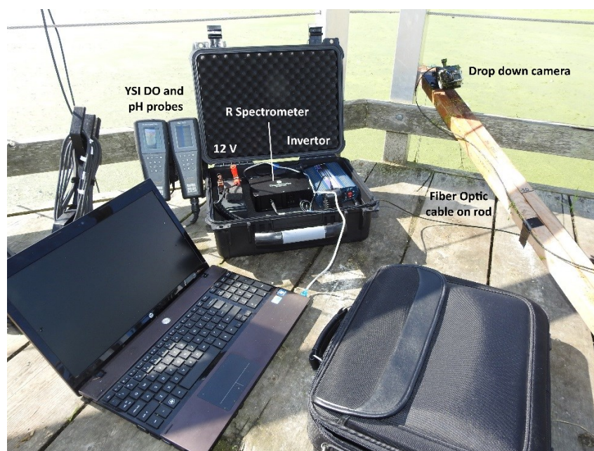
Figure 1. Field configuration of model R Spectrometer used in aquatic light penetration study.
