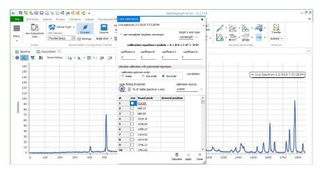
In this case for example, the automatic setting does not detect the structure at 407. But if we lower the threshold to 5% the 407 peak will be detected:
