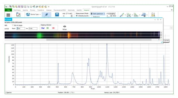
After acquiring an appropriate spectrum, open the calibration dialog from the "*calibr. x* axis" button's drop-down menu.
