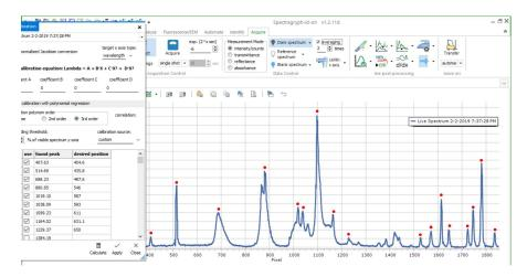
Click on "Calculate" to calculate the new coefficients of the calibration, select always a 3<sup>rd</sup> order for the best results.
