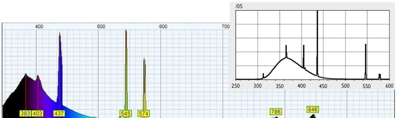
Spectrum of a Philips 6W/05 actinic lamp. Note the great similarity with the characteristics published by Philips (small spectrum at the top-right)
