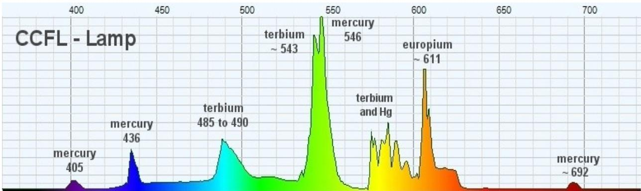
The lines at 436 and 546 nm are accurate. The position of the other rows is not stable and can change from one lamp to another.
