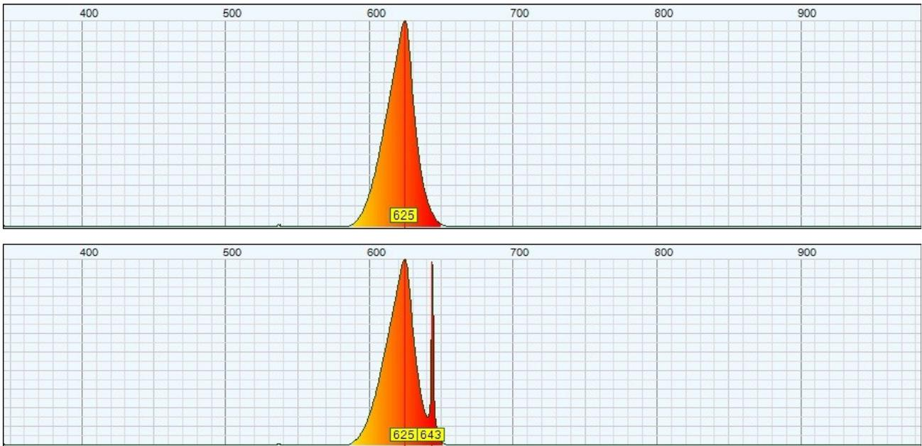
**Red LED + Red Laser.** Note the resolution of the laser line and the line of the red LED is not affected by the laser light, only a few nanometers away.
