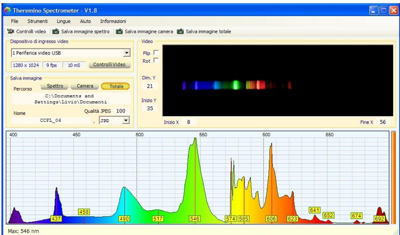
Theremino Spectrometer that displays the spectrum of a fluorescent lamp
