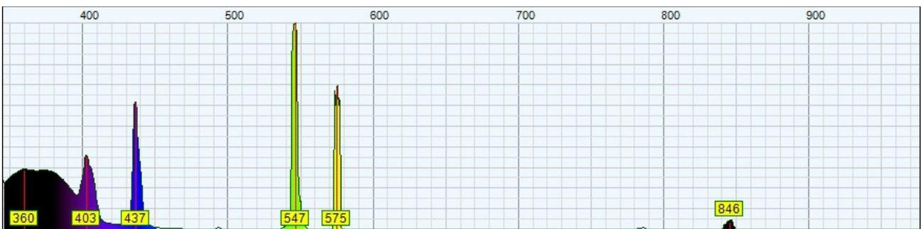
Spectrum of a Philips 15W CLEO tube.
