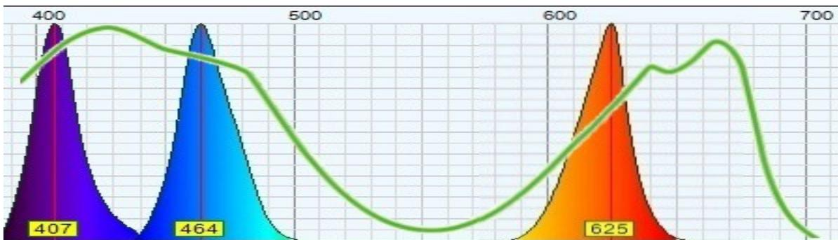
Output of LED ultraviolet, blue, and red superimposed with the photosynthesis efficiency curve
