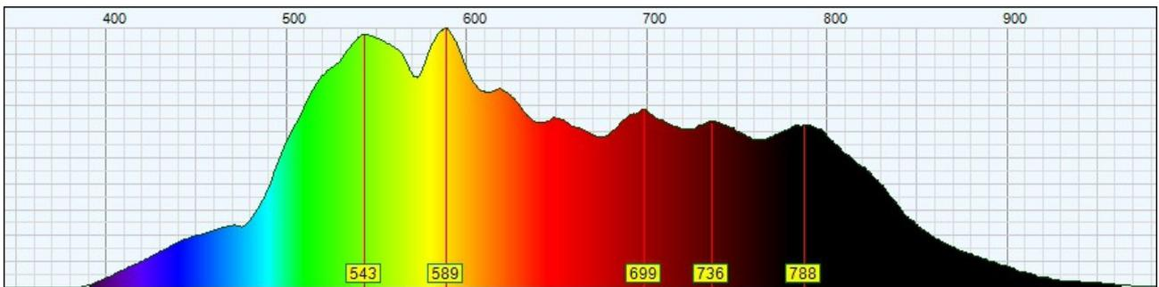
Filament bulbs emit energy across the spectrum in the visible and infrared. The higher the temperature of the filament and the greater the production of visible light, compared to the light "wasted" in the area of the invisible infrared.
